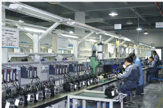
Servo Motor Production Line
