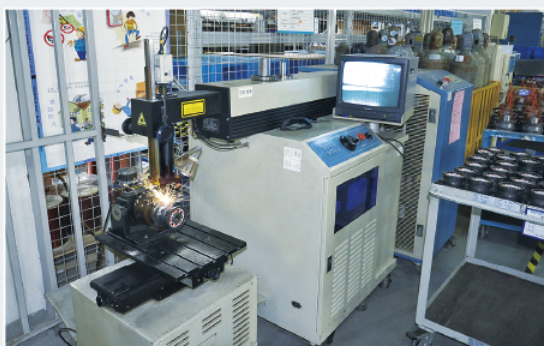
Automatic Laser Welding
